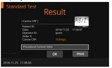
9. Press 'OK' to display the 'Eject Device' screen. The test device can then be removed from the analyzer.
