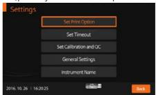
To set the number of printed sheets as 1, 2, or auto-printing mode (ON/OFF), press'Set Print Option'. Check 'Auto Printing' to automatically print all test results at the end of each test.
