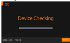
When the procedure for checking the test device is completed, apply the control solution to the sample well of the test device and press 'START' immediately.
