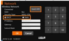
Select the desired WiFi network from the 'Wireless Network' to connect. If a successful connection is made, 'Connected' will be displayed on the top-left corner, and a 'W' mark will appear in the lower-left corner.
