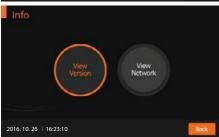
Press 'View Version' to display the version information for the software and firmware. Press 'OK' to confirm.
