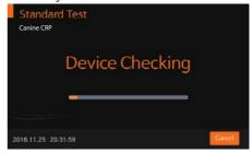
After device checking, apply the specimen to the sample well and immediately press 'START'. If 'START' is not pressed within 20 seconds after applying the specimen, the analyzer will display an error message indicating that the test cannot be performed.
