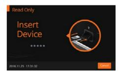
4. Once the test device is inserted into the analyzer, the analyzer will automatically check whether the test device has been used previously or not. The analyzer also reads the barcode data and confirms that the test device is valid before starting the test.
