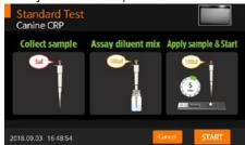
The analyzer will automatically recognize the test device. The time required for analysis depends on type of test device.
