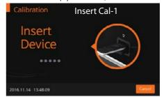
Once the device is inserted into the analyzer, the analyzer will automatically check whether CAL-1 has been used or not. Additionally, the analyzer will read the barcode data and confirm the device validity before starting the calibration set test.
